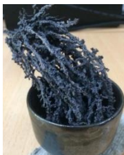
Figure 1. Nickel ferrite ( \text{NiFe}_2\text{O}_4 ) obtained by sol-gel autocombustion method
